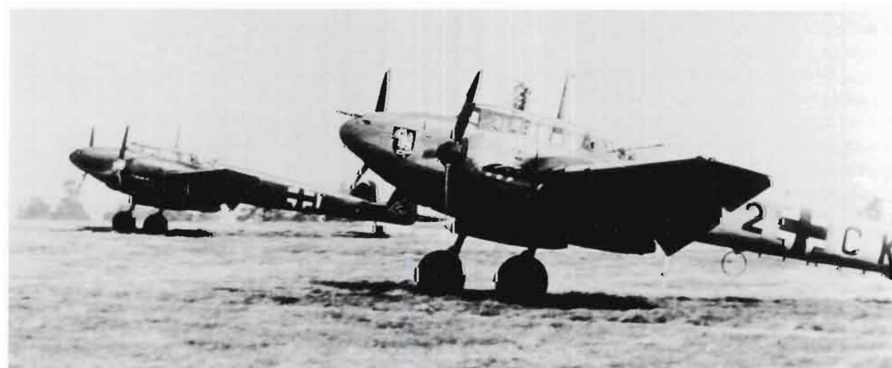
RIGHT: Lt. Horst Marx, a pilot of 3./Erp. Gr. 210, with a Bf 110 D-0 'Jabo' of Erp. Gr. 210 as a backdrop in this photograph. This aircraft is probably from the first batch issued to the unit, as it carries the solid two-tone upper surface camouflage. The unit emblem, and the extended rear fuselage of the 'D' variant can be seen.
