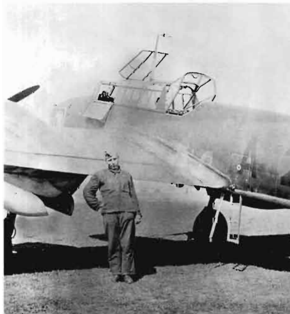
LEFT: An unknown ground mechanic poses in front of a Bf 110 C of I./ZG 52 . Note the fully enclosed Bordfunker's central rear canopy. Seen to good effect are the first aid hatch, the ladder for access to the port wing, and the aerial beside it.
