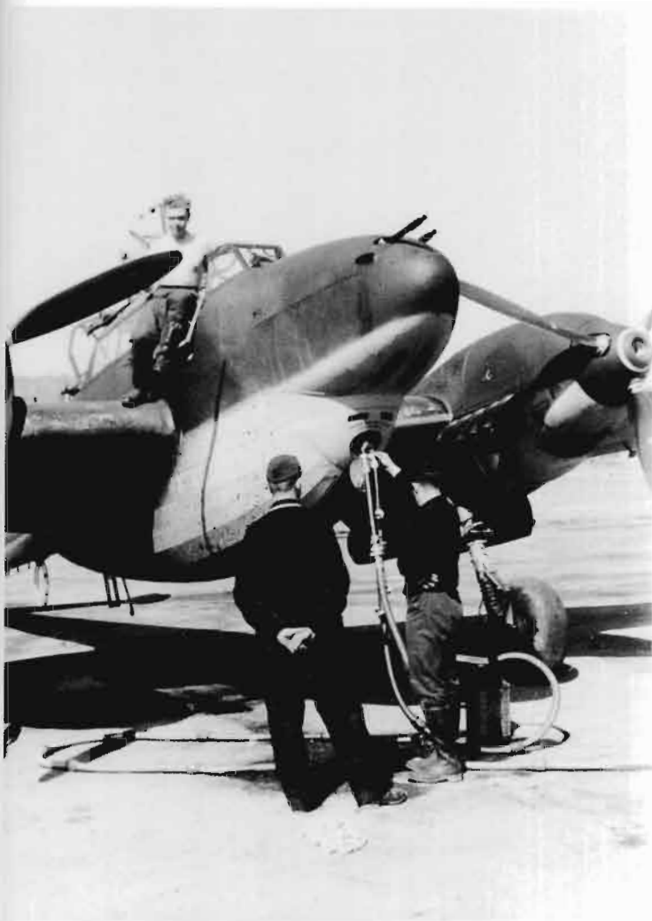
BELOW: The front view of a Dackelbauch of 1./ZG 76 being re-fuelled. Note the re-fuelling point in the front centre of the Dackelbauch.
