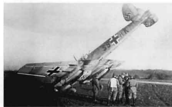
ABOVE: An ignominious nose-over in soft ground for S9+HK, a Bf 110 D of 2./ Erpr. Gr. 210 . This view shows the fuselage bomb rack to good effect.
