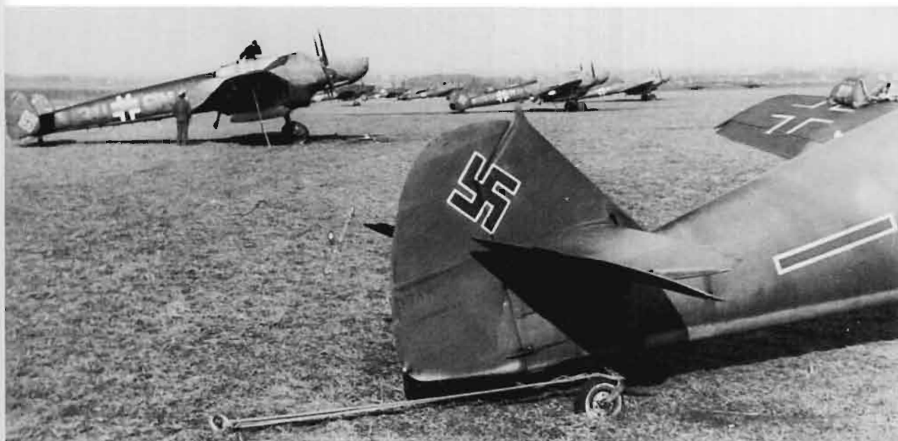
LEFT: Covers are still on the front canopies and noses of these Bf 110 'B' variants of ZG 26. Of note is the early style camouflage, but the whole of the swastika on the fin was somewhat uncommon on 'B' series aircraft; it was more commonly seen across both fin and rudder.
