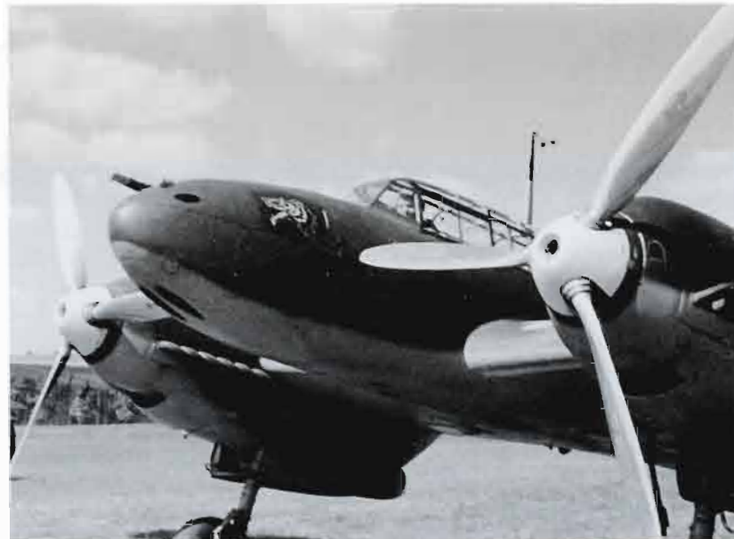
ABOVE: A close-up of the nose of L1+A11 showing the unit emblem and white spinner caps. The propeller blades appear to be wooden.
