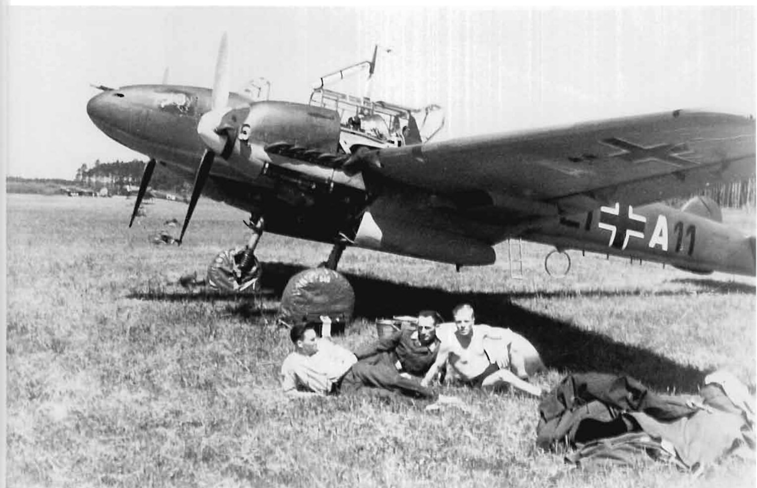
ABOVE AND RIGHT: This Bf 110 C-1, 11+A11, of 1.(schwere Jagd)/LG 1 carries the earliest style of unit markings on the fuselage. Note the two antennae coming from the cockpit aerial mast, the Gruppe emblem on the nose and the thin underwing cross placed near the wingtip. This 'C' also has the rounded wingtips common to the 'B' variant which would change to 'squared-off' wingtips as the 'C' variant developed.
