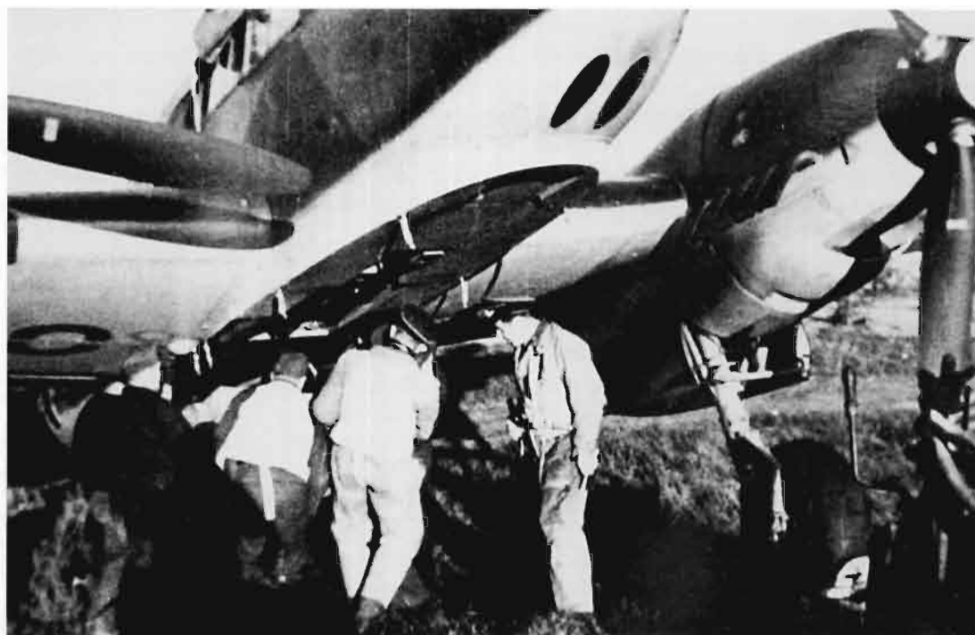
RIGHT, BELOW AND BELOW RIGHT: Three views showing a Dackelbauch being fitted to a Bf 110 D of I./ZG 76. Note the individual aircraft letter, G, on the nose, and the fuel staining on the front of the ribbed fairing.
