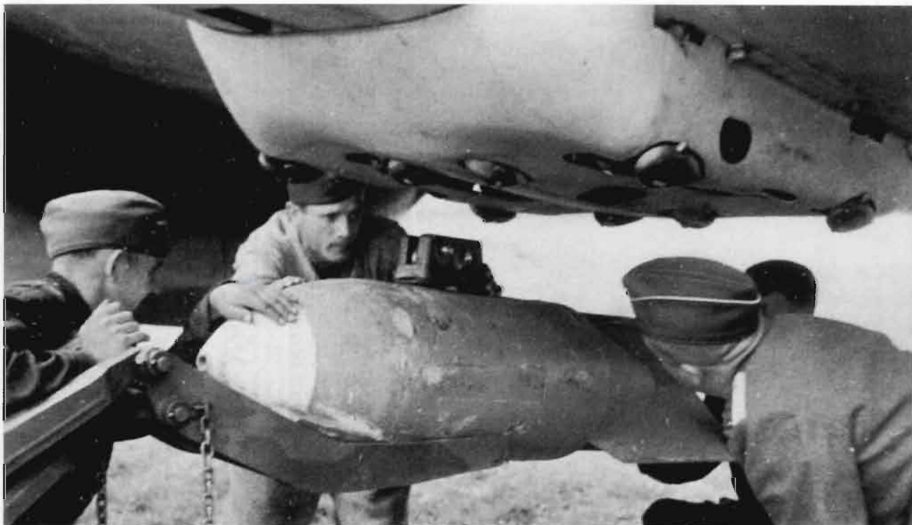
RIGHT: Mechanics fit a bomb onto the fuselage bomb rack of a 'Jabo' of Erpr. Gr. 210.
