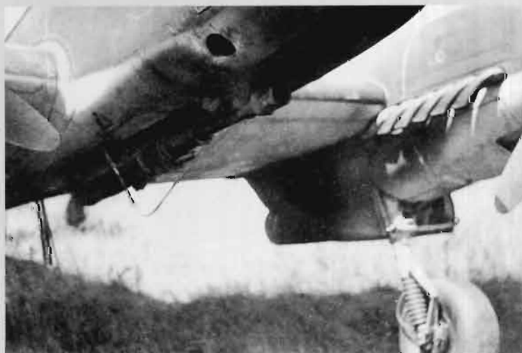
BELOW: The 30 mm Kanone installation with the fairing removed.
