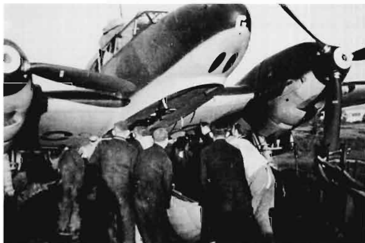
RIGHT, BELOW AND BELOW RIGHT: Three views showing a Dackelbauch being fitted to a Bf 110 D of I./ZG 76. Note the individual aircraft letter, G, on the nose, and the fuel staining on the front of the ribbed fairing.
