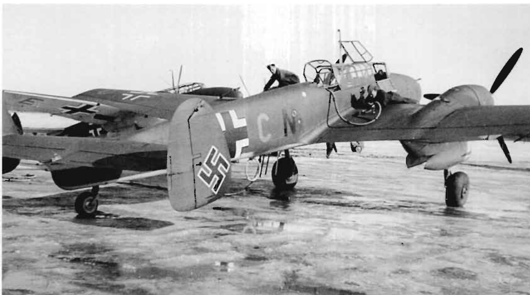
LEFT: 2N+CN of 8./ZG 76 having its wing fuel tanks replenished. This aircraft has the initial style Bordfunker's central enclosed panel, which required it to be partially opened for the Bordfunker to swing the machine gun into the firing position. The individual aircraft letter 'C' is in red and unusually, it is also in red on the top surface of the port wing.
