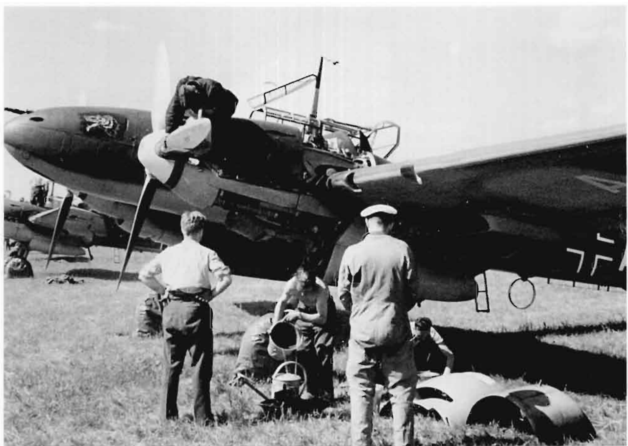
ABOVE AND RIGHT: This Bf 110 C-1, 11+A11, of 1.(schwere Jagd)/LG 1 carries the earliest style of unit markings on the fuselage. Note the two antennae coming from the cockpit aerial mast, the Gruppe emblem on the nose and the thin underwing cross placed near the wingtip. This 'C' also has the rounded wingtips common to the 'B' variant which would change to 'squared-off' wingtips as the 'C' variant developed.
