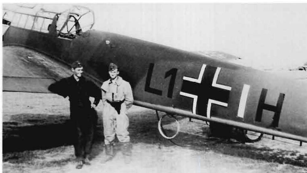
LEFT: L1+IH, a Bf 110 C-1 of 13.(Z)/LG 1 displays the aerial attachment point on the port side of its fuselage. Note the fully enclosed type of rear central panel for the Bordfunker.
