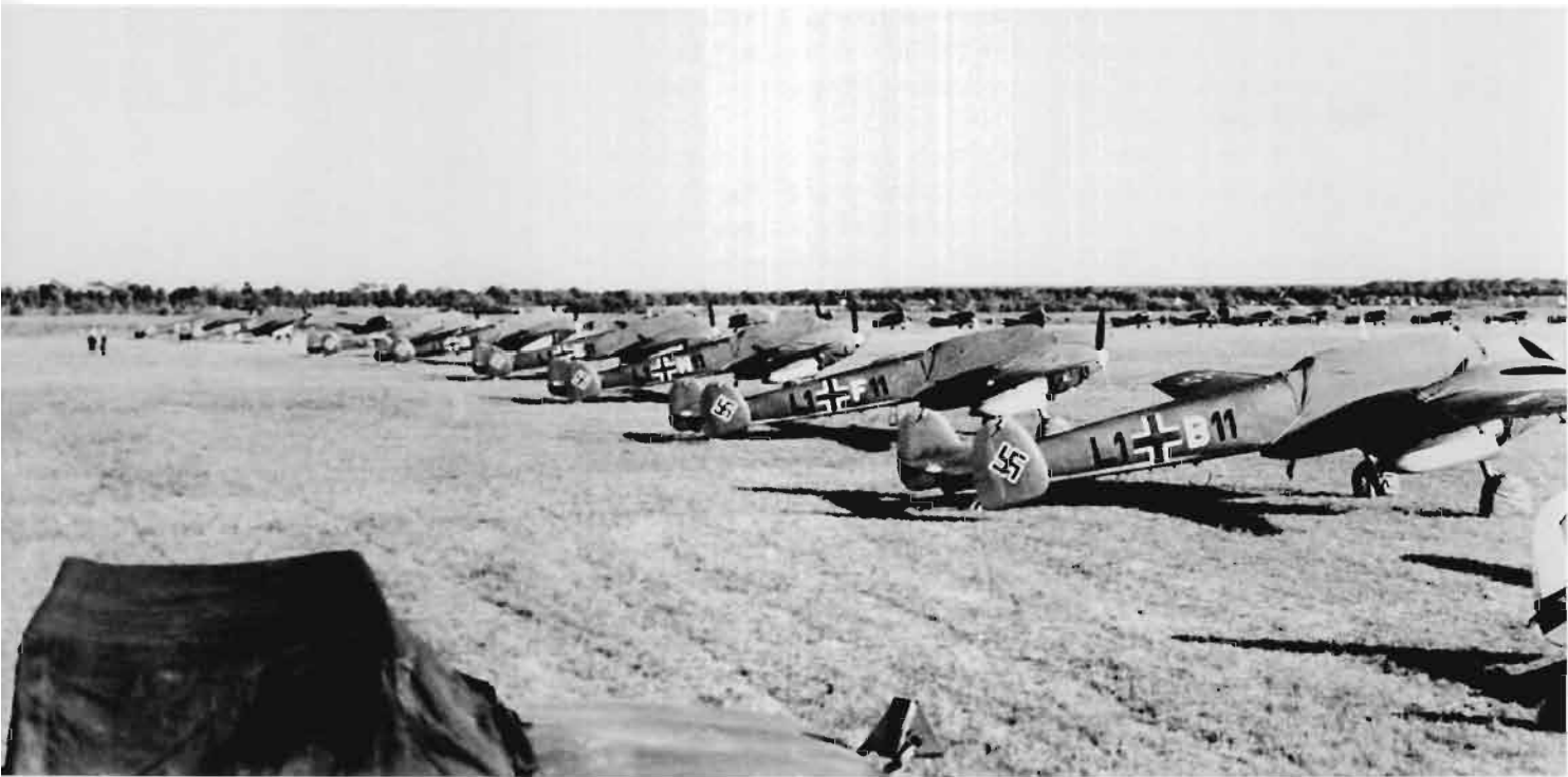
THIS PAGE: A line-up Bf 110s of I.(schwere Jagd)/LG 1 sporting the early fuselage codes at Barth in the summer of 1939. Protective covers on the cockpits, the early style thin fuselage cross and the swastika across both fin and rudder can be seen.
