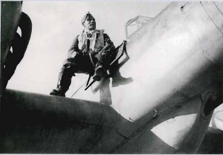
ABOVE: Balthasar Aretz sits on the cockpit sill of this Bf 110 C-6 of 1./Erpr. Gr. 210. Note the hinge on the starboard side of the fairing allowing the housing to swing down for servicing and maintenance of the 30 mm. Kanone.
