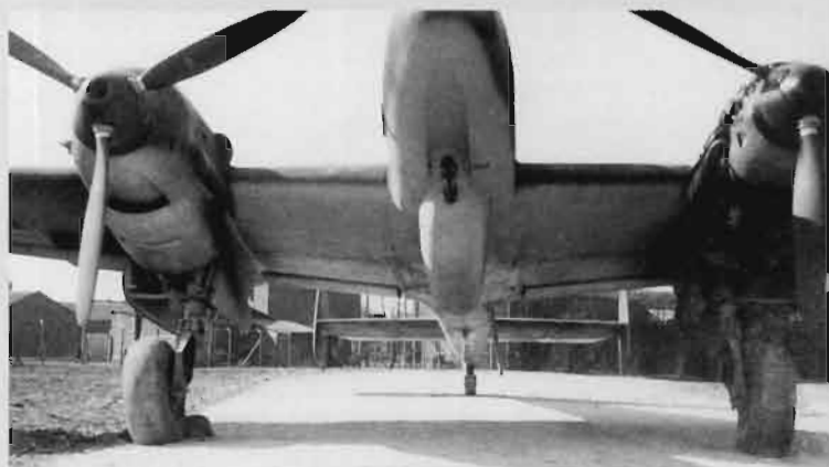
ABOVE: A head-on view of the 30 mm MG 101 Kanone fitted to a Bf 110 C-6 of 1./ Erpr. Gr. 210 .
