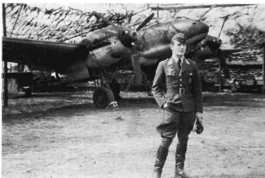
RIGHT: Lt. Horst Marx, a pilot of 3./Erp. Gr. 210, with a Bf 110 D-0 'Jabo' of Erp. Gr. 210 as a backdrop in this photograph. This aircraft is probably from the first batch issued to the unit, as it carries the solid two-tone upper surface camouflage. The unit emblem, and the extended rear fuselage of the 'D' variant can be seen.
