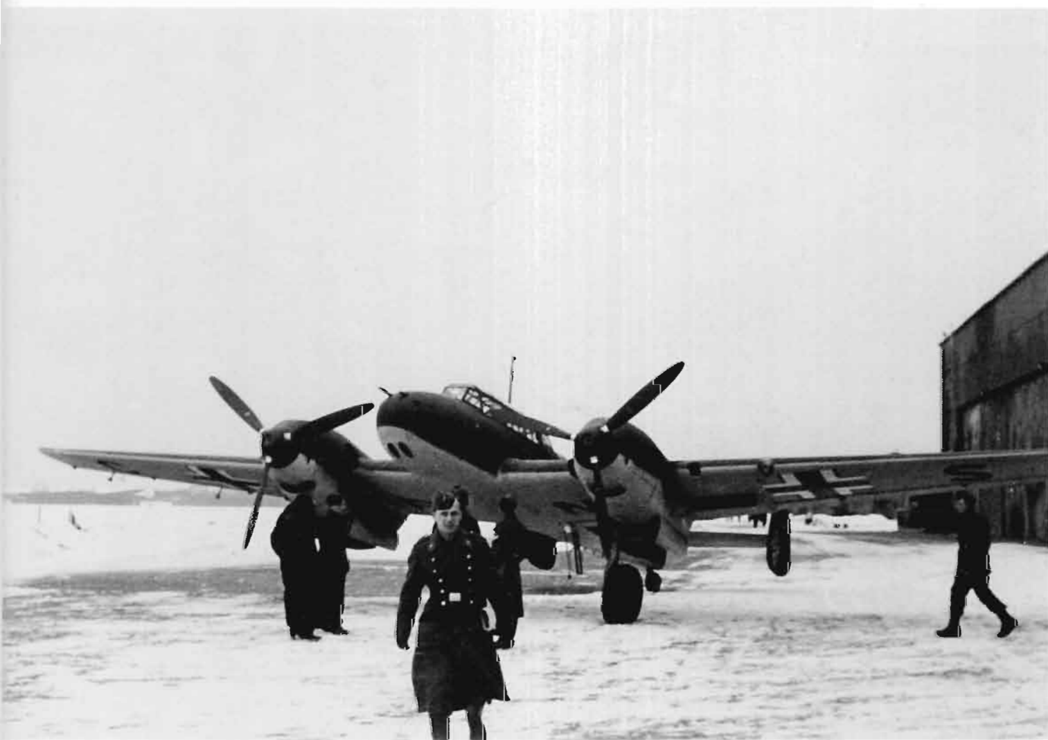
BELOW: This C-2 in a wintry scene still carries the Stammkennzeichen on the undersides of the wings. The early style solid upper surface camouflage can be clearly seen and the swastika is carried on the fin only.
