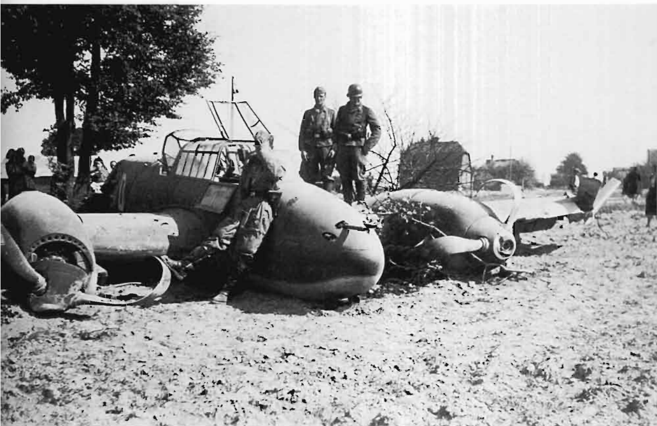
LEFT: The pilot of this Bf 110 C-1 has made a relatively good belly-landing, although it appears that the aircraft finally came to rest with the aid of the tree. This aircraft carries the early style fuselage cross with the thin white area and the fully enclosed Bordfunker's rear canopy. The cockpit canopy antenna clearly has two aerial leads hanging from it, denoting the early radio system fitted to 'B' and 'C-1' series Bf 110 aircraft. The spinner tips have a single ring around them, which, like the individual aircraft letter 'D', appear to be white.
