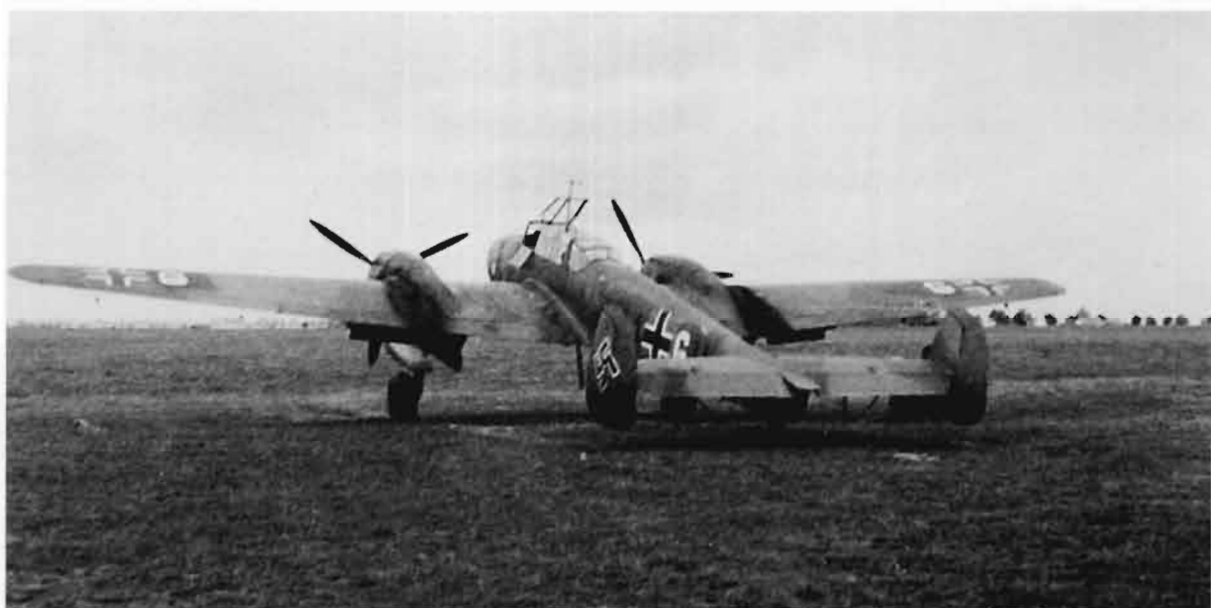
RIGHT: Bf 110 C-1, L1+GH of 13.(Z)/LG 1. This machine carries the early style fuselage cross and has its individual aircraft letter, 'G' inboard of the upper surface wing cross.
